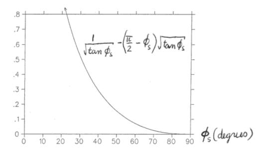
**Ex:** At mid-cycle in the SSC LEB,  $T = (\gamma - 1)\mathcal{E}_0 = 5.73 \text{ GeV}, \delta \mathcal{E} = 0.611 \text{ MeV}$ (comes from a total energy gain of 10.5 GeV in a sinusoidal acceleration ramp of 50 ms). For  $\epsilon_{\phi} = 0.02 \text{ eVs}$  and  $P_f < 0.5$ , find the upper limit on  $\phi_s$  and the lower limit on V. Ans: 52° and 770 kV.
