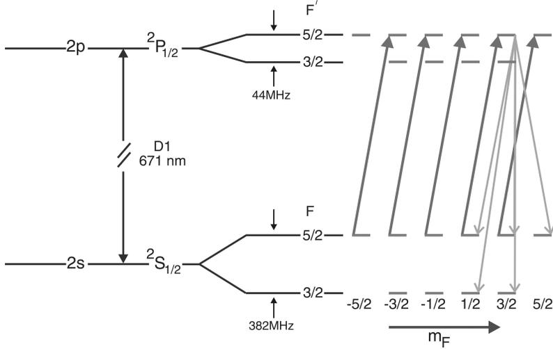
Fig. 2. Optical pumping scheme for polarized  ${}^8\text{Li}$ . For clarity, the optical transitions from the  ${}^2S_{1/2}, F = 3/2$  to the  ${}^2P_{1/2}, F = 5/2$  are not shown.
