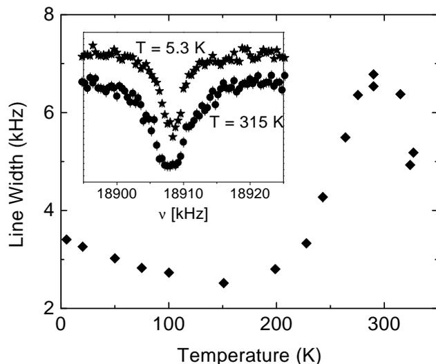
Fig. 3. The inset shows the resonances in GaAs at two temperatures. The main part shows the temperature dependence of the linewidth.
