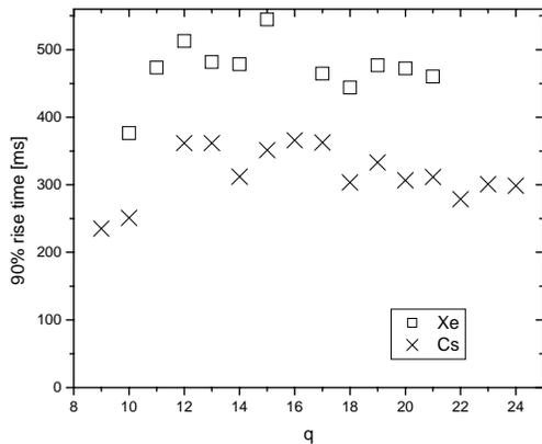
Figure 2 time to reach 90% of the signal after pulsed injection of singly charged ions
