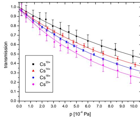
Figure 3 Transmission of  $Cs^{10+}$ ,  $Cs^{14+}$ ,  $Cs^{18+}$  and  $Cs^{23+}$  as function of  $N_2$  pressure, together with fitted curves
