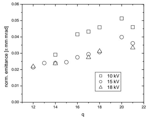
Figure 1 normalized emittance of highly charged Cs beams at several extraction voltages.
