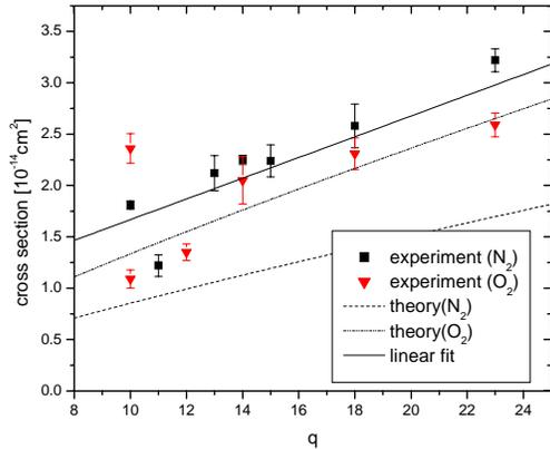
Figure 4 Experimental cross sections for the charge exchange of Rb and Cs ions in N<sub>2</sub> and O<sub>2</sub> gas together with the expectation from equation 1 and a linear fit. The error bars only represent statistical errors.
