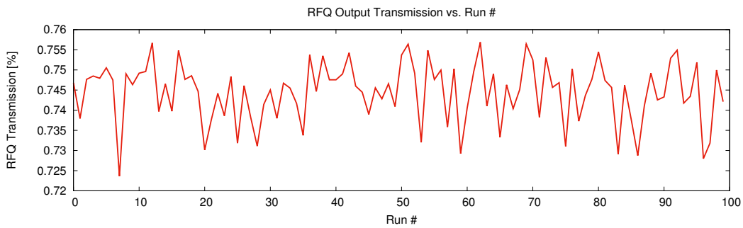
Figure 7: Simulated RFQ Transmission of 100 PARMELA/PARMTEQ runs with \pm 1\% , 1^\circ Monte-Carlo sampling for voltage and phase, respectively.
