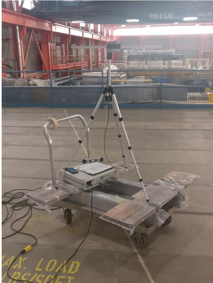
Figure 11: Axially symmetric measurement experimental set-up of tripod jig and other tools on a mobile platform, and a tape alignment line on the ground.
