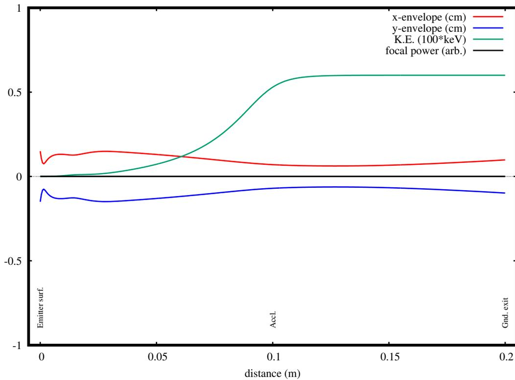
Figure 10: Calculated beam envelope for the 60 keV  $^{133}\text{Cs}^+$  ion beam through the extraction system.
