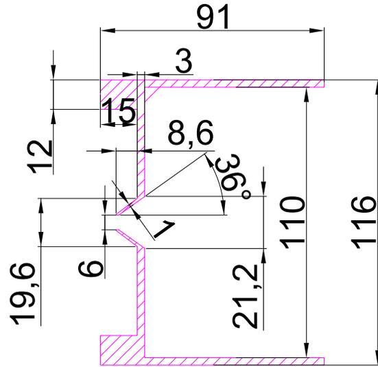
Figure 5: Layout of the extraction electrode. Remove sharp corners by fillet with radius about 0.25 mm.
