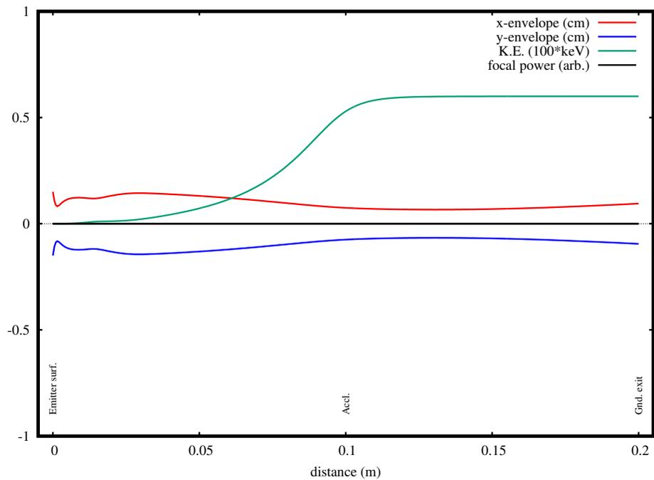
Figure 12: Calculated beam envelope for 100 nA 60 keV  $^{133}\text{Cs}^+$  ion beam through the extraction system.
