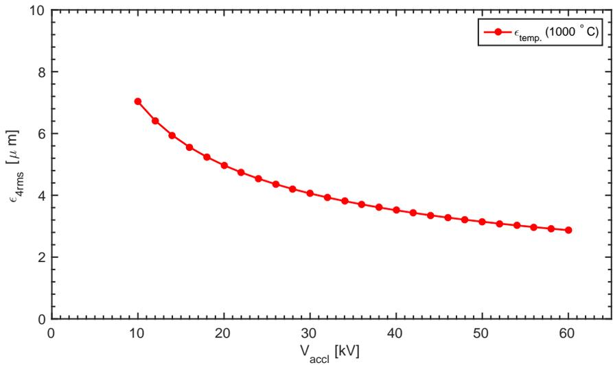
Figure 7: Calculated 4rms emittance of  $^{133}\text{Cs}^+$  ion beams due to thermal temperature about  $1000^\circ\text{C}$  at various acceleration potential of the extraction system.
