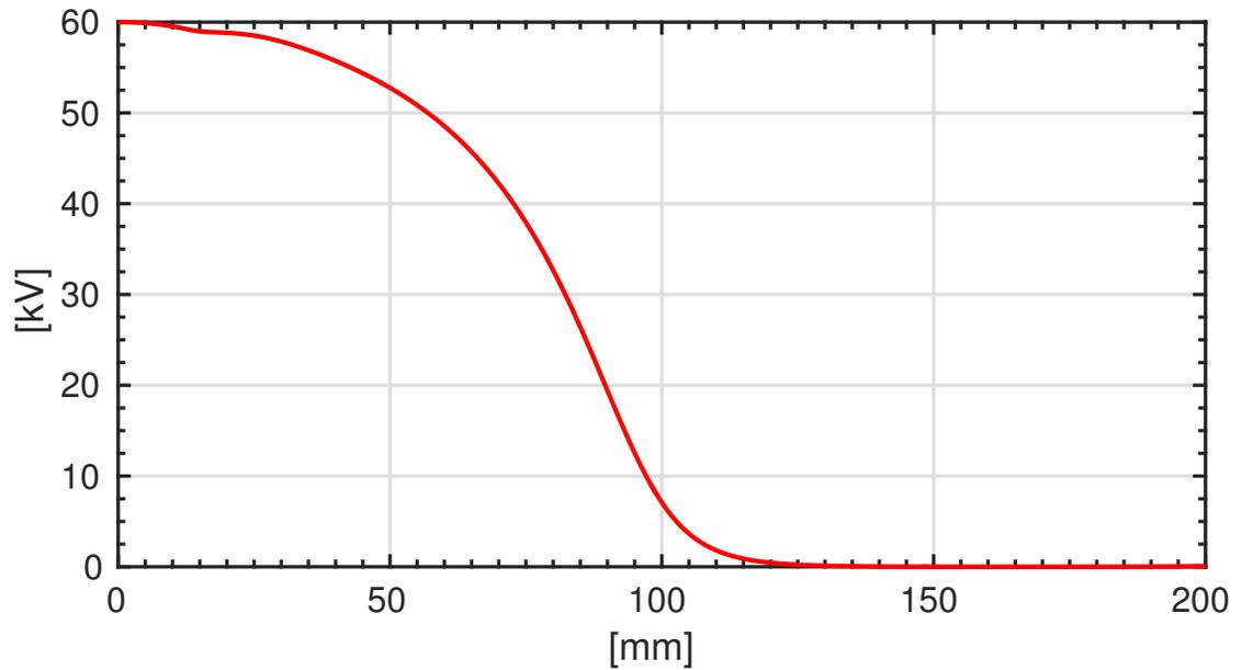
Figure 9: Calculated potential along the axis of the extraction system.
