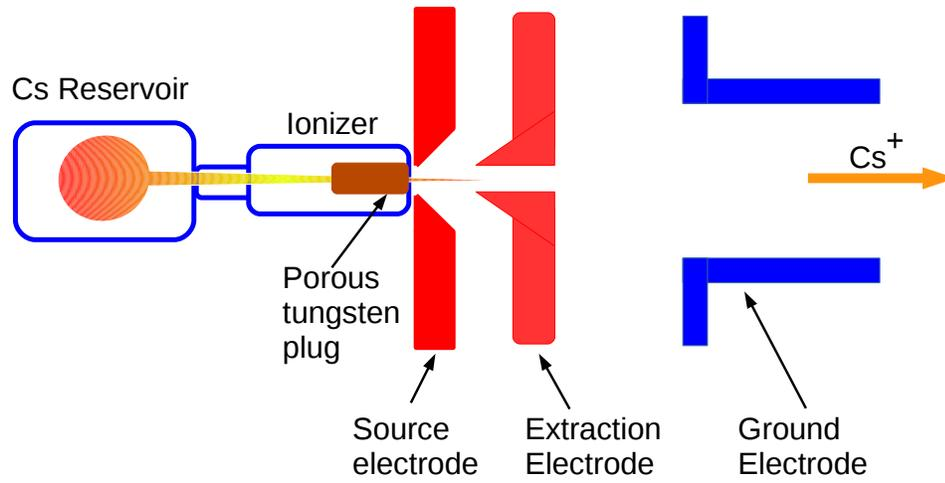
Figure 1: A schematic view of a surface ion source for  $\text{Cs}^+$  beams.
