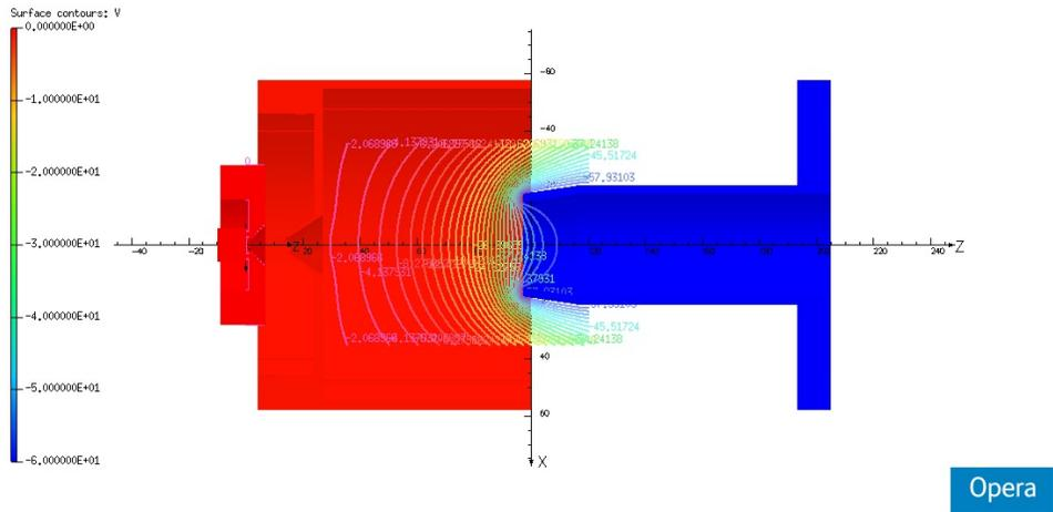
Figure 8: Equipotential contour in the xz plane of the extraction system.
