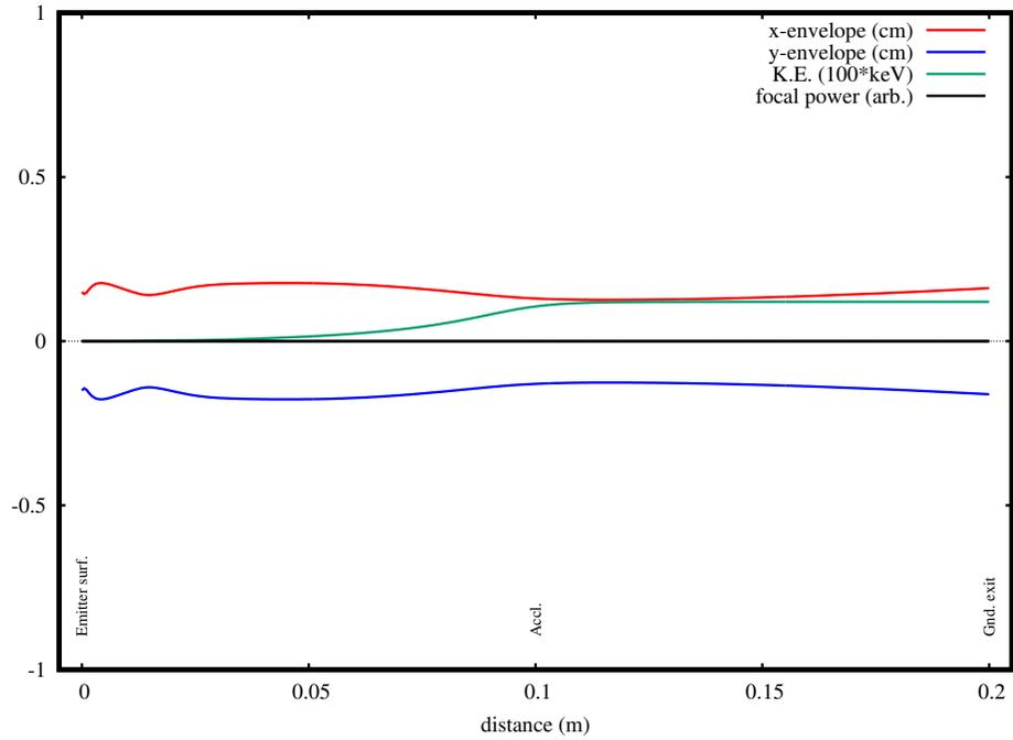
Figure 11: Calculated beam envelope for the 12 keV  $^{133}\text{Cs}^+$  ion beam through the extraction system.
