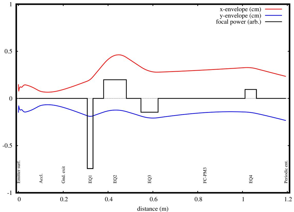
Figure 13: Calculated beam envelope for the 60 keV  $^{133}\text{Cs}^+$  ion beam through the extraction and beam transport systems.
