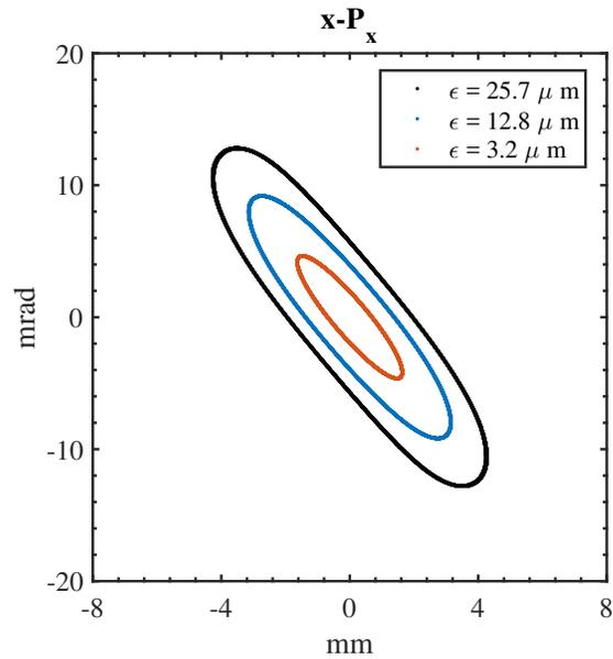
Figure 14: Calculated phase-space profiles by using the code COSY INFINITY for various beam emittances in the horizontal plane at the entrance of a periodic section in the ARIEL RIB beamline.
