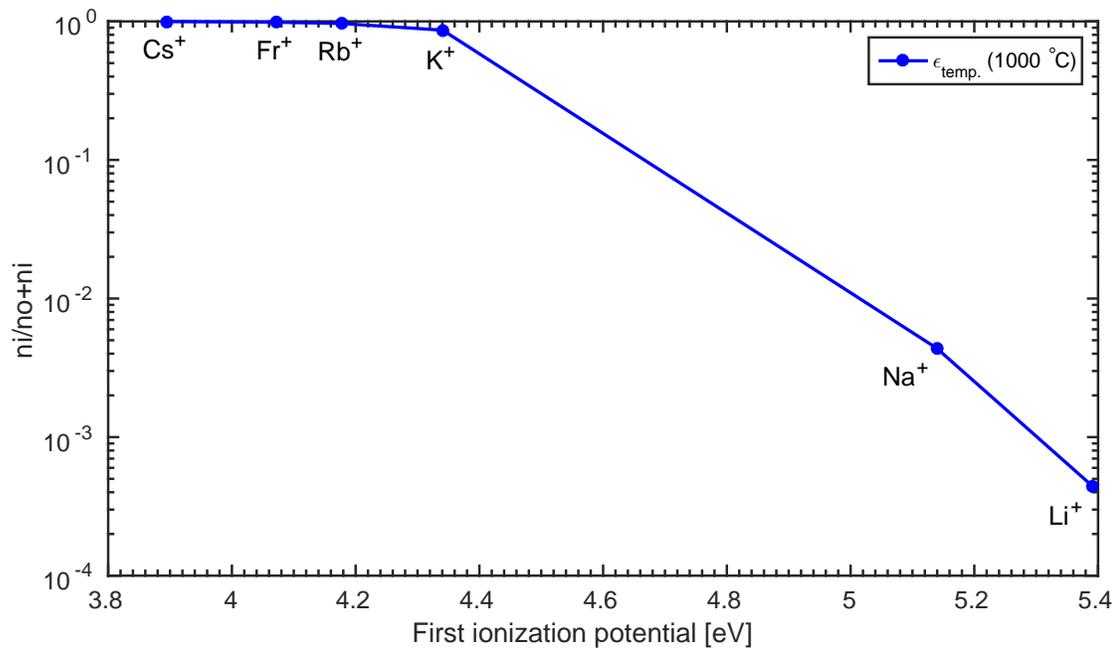
Figure 2: Calculated ionization efficiency for various alkali elements through a tungsten ionizer with a temperature about  $1000^\circ\text{C}$ .
