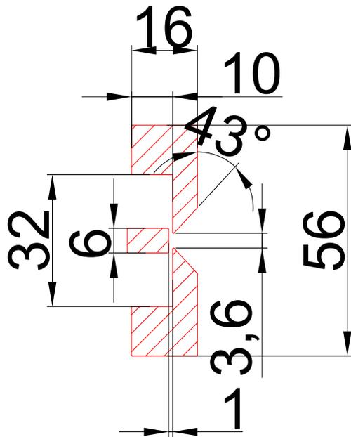
Figure 4: Layout of the source electrode. Remove sharp corners by fillet with radius about 0.25 mm.
