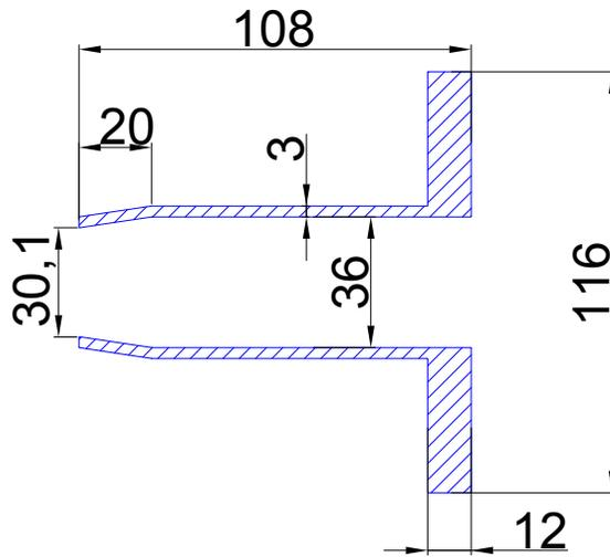
Figure 6: Layout of the ground electrode. Remove sharp corners by fillet with radius about 0.25 mm.
