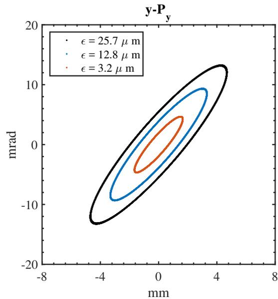
Figure 15: Calculated phase-space profiles by using the code COSY INFINITY for various beam emittances in the vertical plane at the entrance of a periodic section in the ARIEL RIB beamline.
