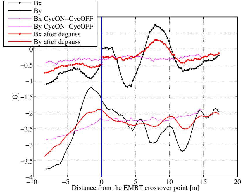
Figure 1: Measurements, before (black) and after (red) demagnetizing.
