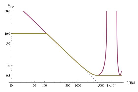
Note the minimum at 3.7 kHz. The curve swings upward at frequencies beyond this, oscillating between infinity and 0.5 Volt. This is due to resonance effects; we cannot take advantage of this because the frequency is not in our control and we would not be able to lock it. Thus, for f > 3.7 kHz, the condition remains at  $V_{\rm p-p} < 0.5$  Volt, as in the brown curve.
