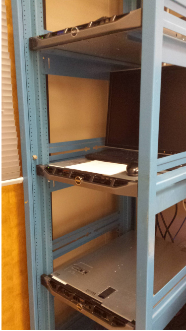
(a) Server rack showing all three stand-alone servers.
