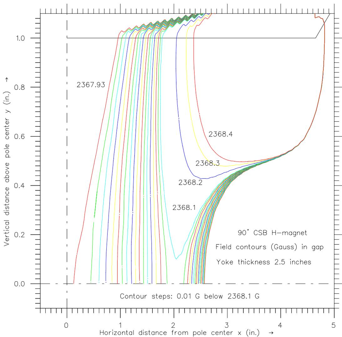
Fig. 6. Field contours in the gap of the CSB 90° dipole with 2.5 inch yoke thickness.
