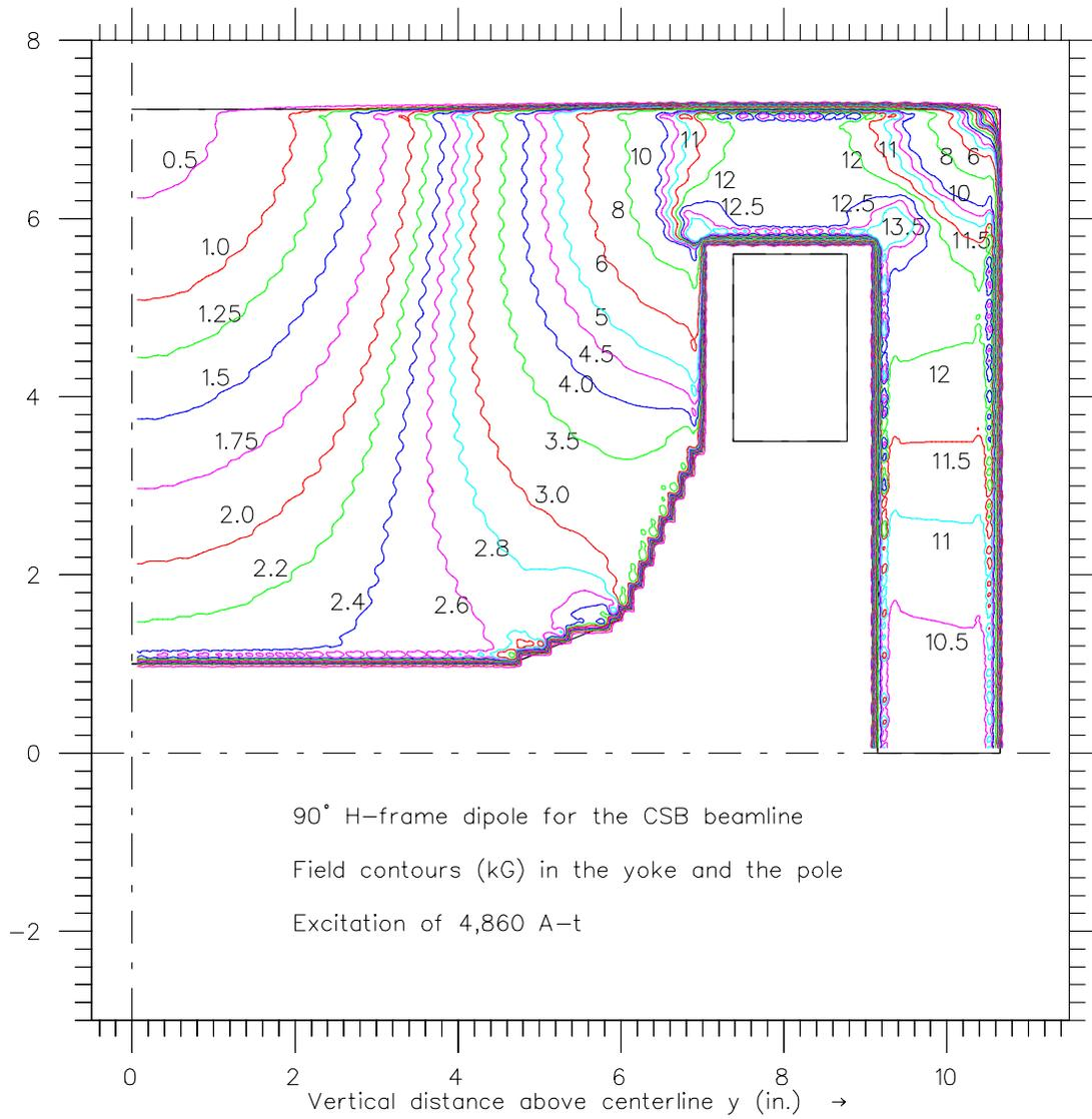
Fig. 3. Field contours in the yoke and pole of the CSB 90° dipole with 1.5 inch yoke thickness.
