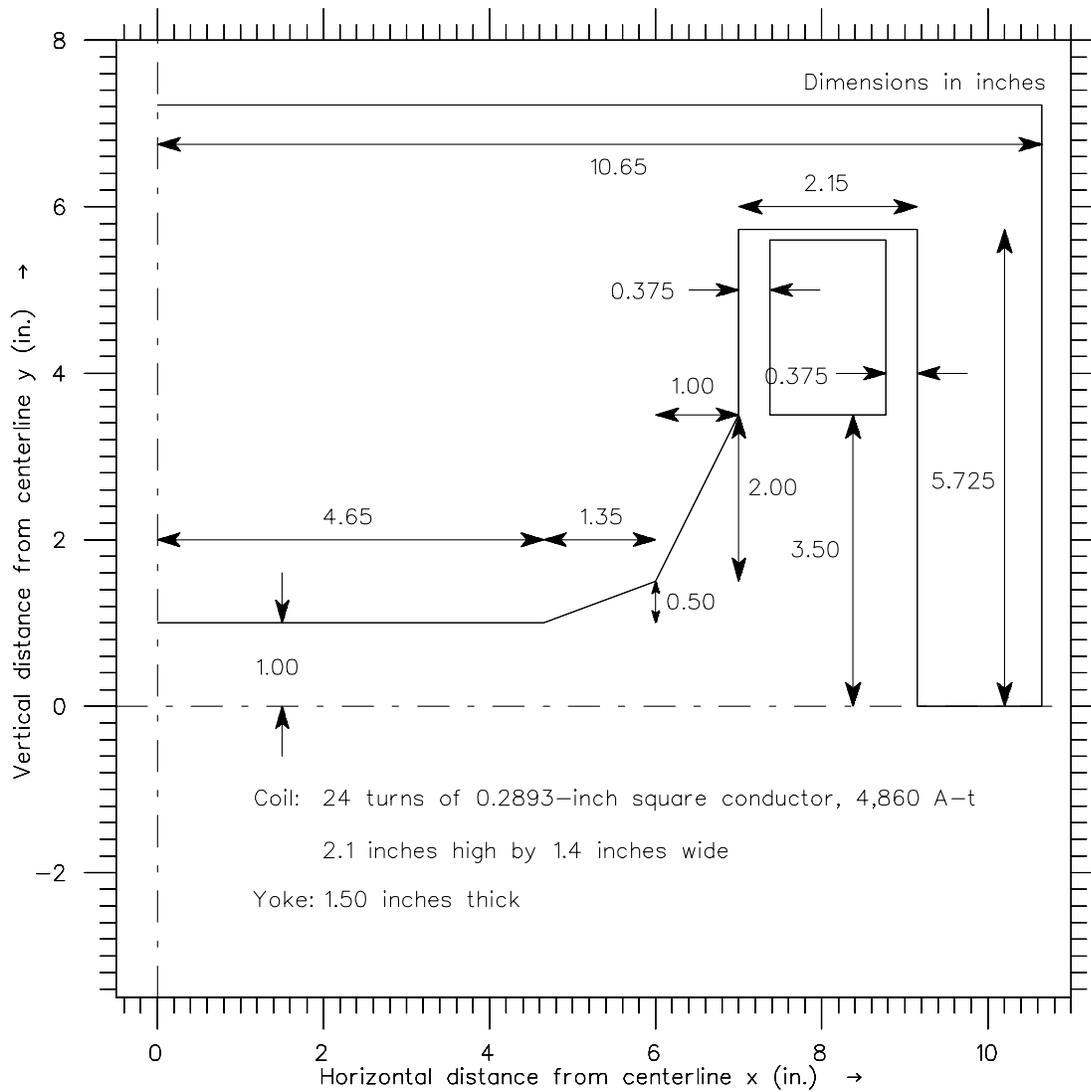
Fig. 1. Quarter-section cross-section of the 90° CSB dipole.
