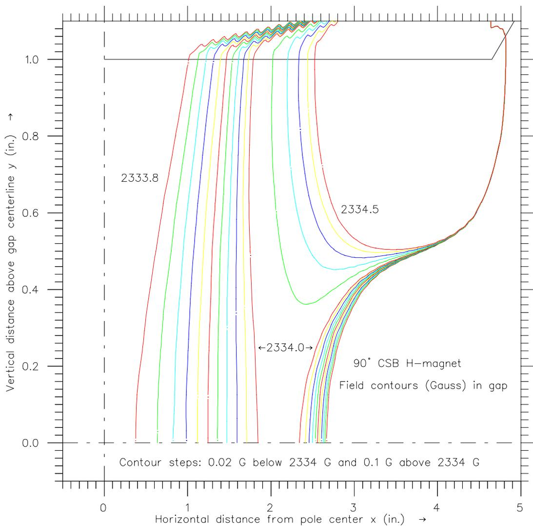
Fig. 4. Field contours in the gap of the CSB 90° dipole with 1.5 inch yoke thickness.
