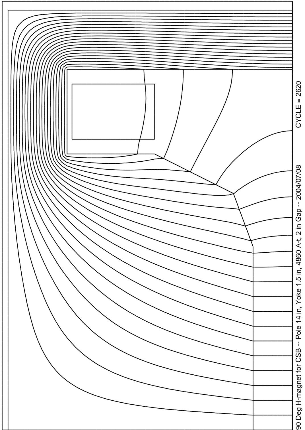
Fig. 2. Illustration of flux concentration in connection between the yoke and the pole.
