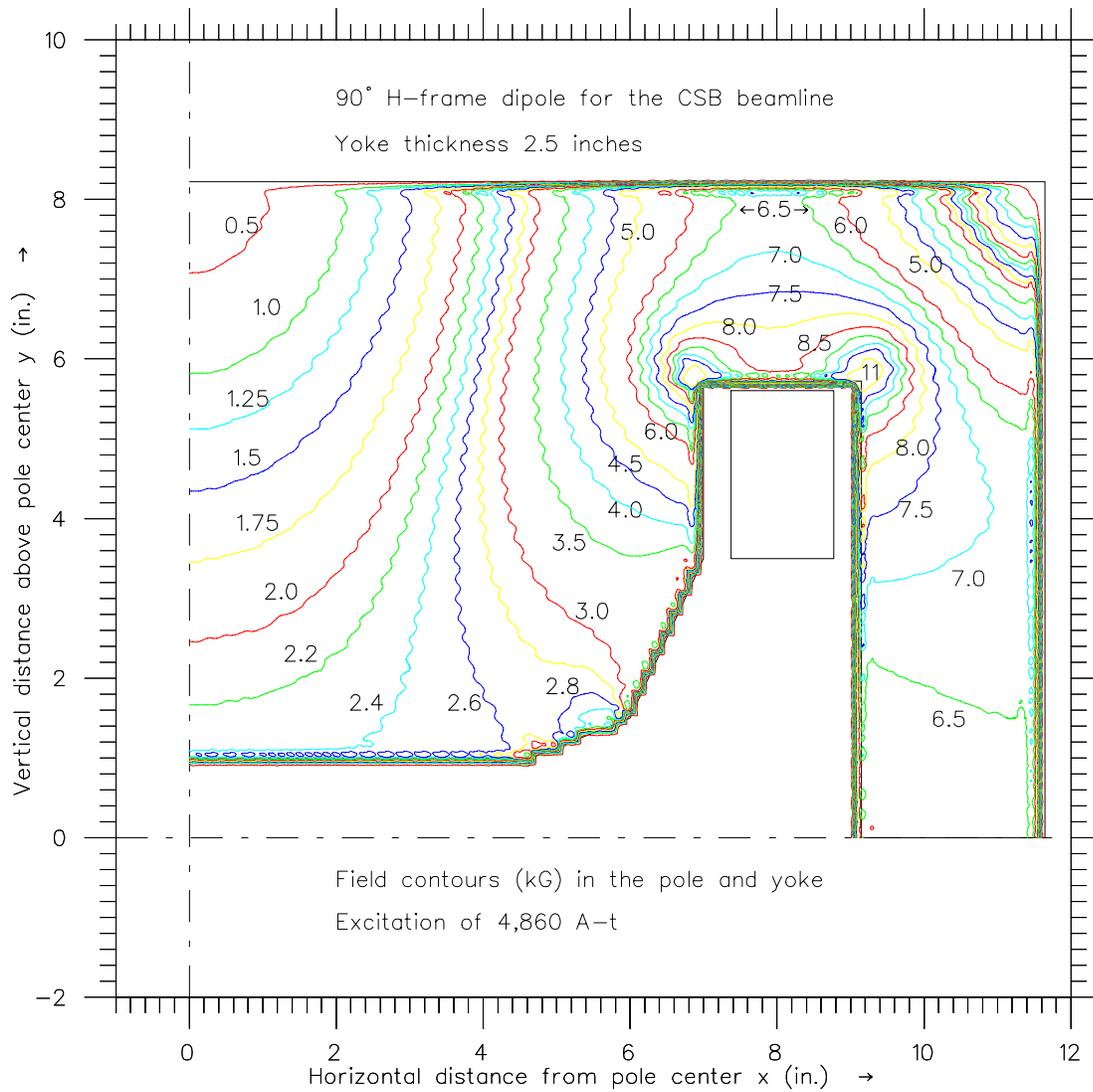
Fig. 5. Field contours in the yoke and pole of the CSB 90° dipole with 2.5 inch yoke thickness.
