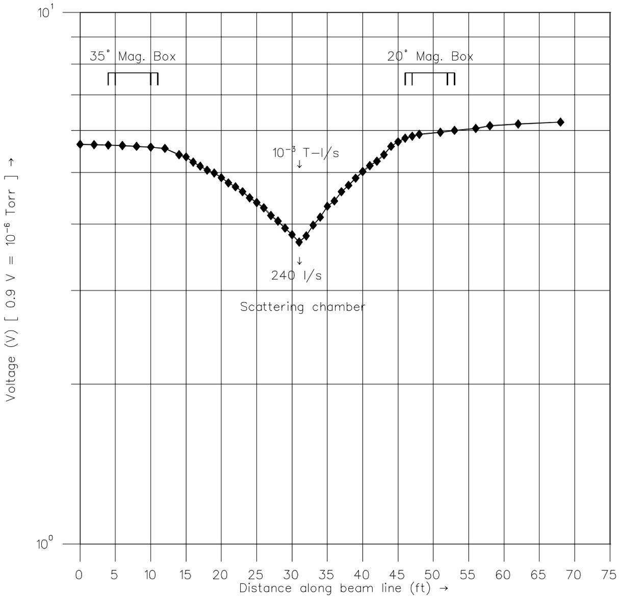
Fig. 5. Beam Line IV-A from LD<sub>2</sub> target to beam dump, pumping at the scattering chamber only.
