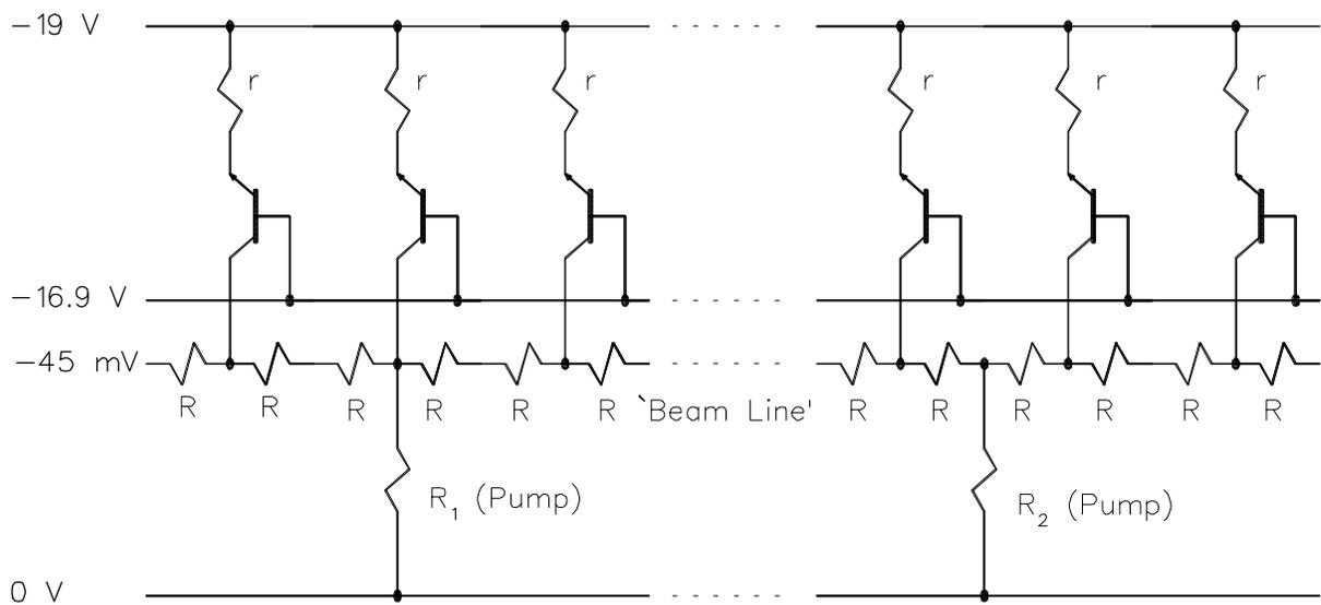
The machine pressure is defined by holding the 'Beam line' at  $45\text{ mV}$ .
