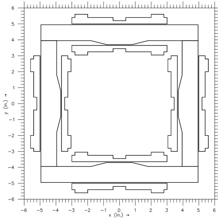
Fig. 2-a. Cross-section of the proposed steering magnet of ref<sup>1)</sup>.
