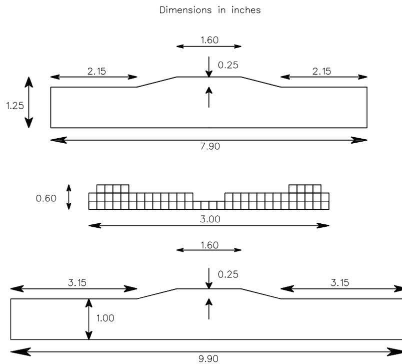
Fig. 2-b. Dimensions of the proposed steering magnet components of ref<sup>1)</sup>.
