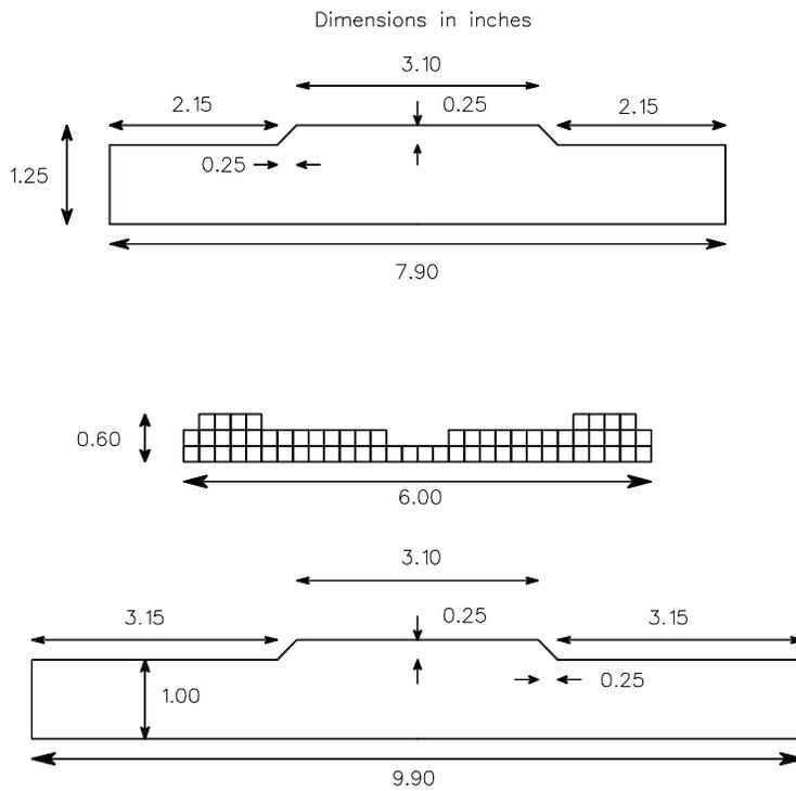
Fig. 1-b. Dimensions of the proposed steering magnet components.
