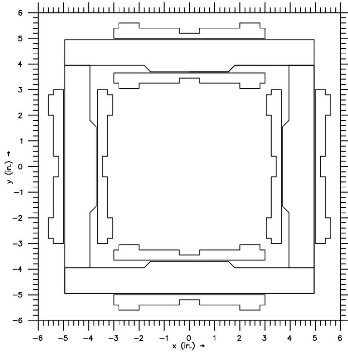
Fig. 1-a. Cross-section of the proposed steering magnet.
