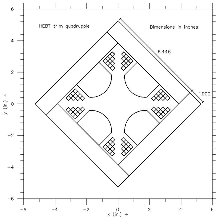
Fig. 8. Overall dimensions of this HEFT quadrupole.
