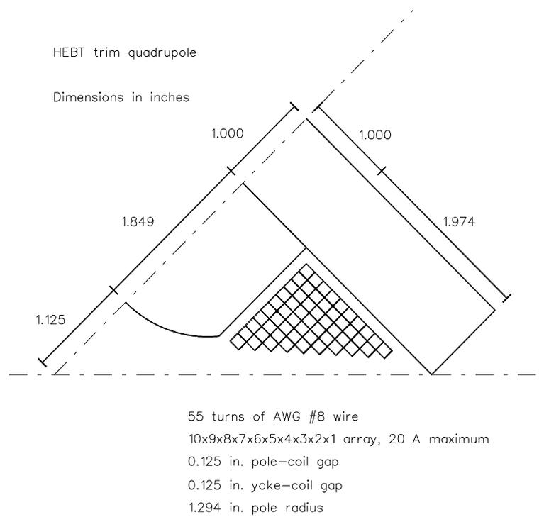
Fig. 2. An octant of a HEFT quadrupole with a coil of 55 turns of AWG #8 wire.
