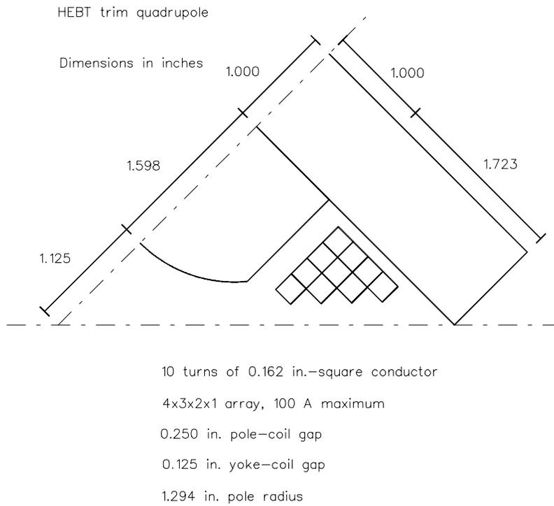
Fig. 7. An octant of a HEFT quadrupole with a coil of 10 turns of 0.162 in. square conductor.
