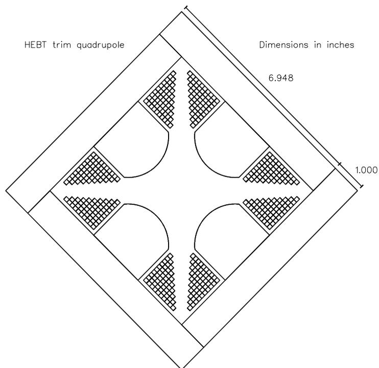
Fig. 3. Overall dimensions of this HEFT quadrupole.
