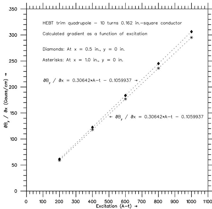
Fig. 11. Calculated gradient as a function of excitation of a HEBT quadrupole with a coil of 10 turns of 0.162 in. square conductor.
