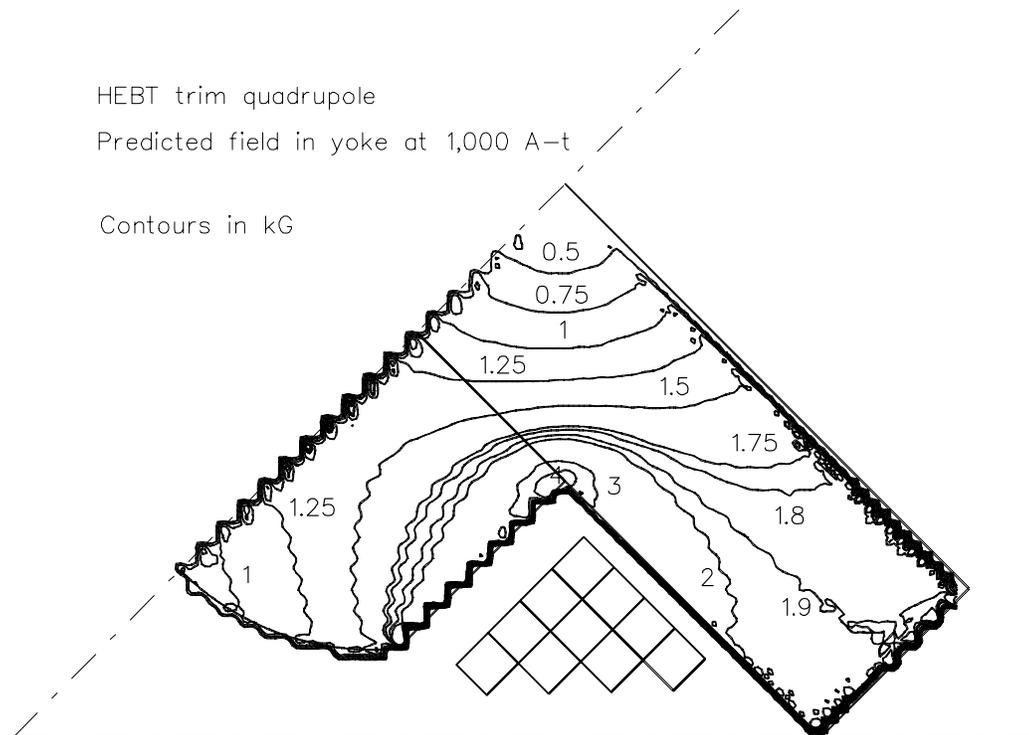
4x3x2x1 array of 0.162 in.-square conductor
