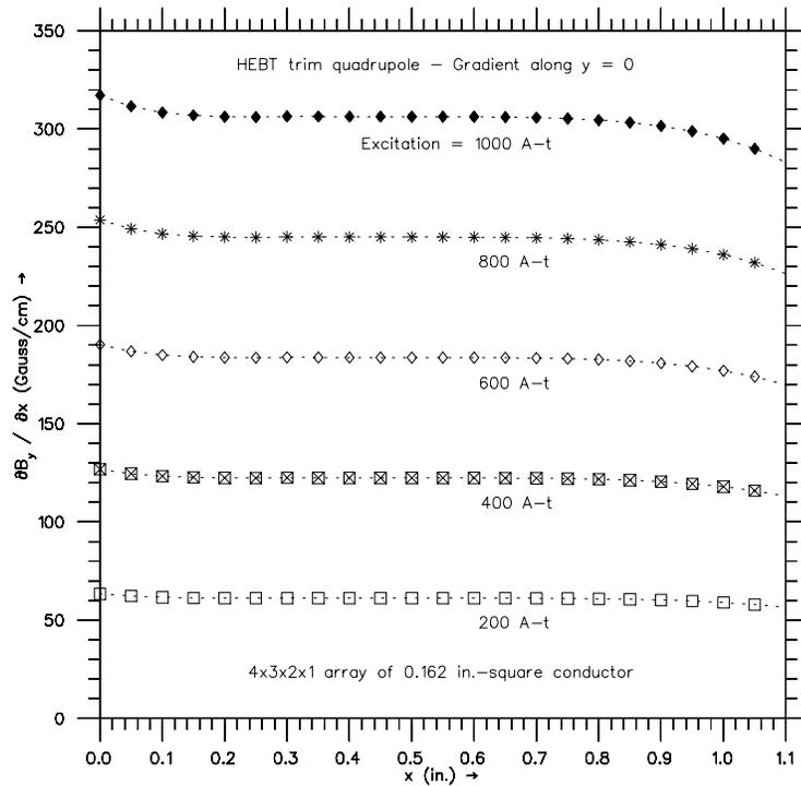
Fig. 10. Calculated gradient as a function of radius and excitation of a HEBT quadrupole with a coil of 10 turns of 0.162 in. square conductor.
