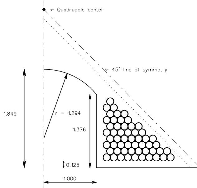
Fig. 1. Coil and yoke cross-sections for AWG #8 wire. Dimensions are inches.
