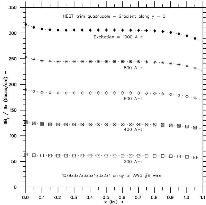
Fig. 5. Calculated gradient as a function of radius and excitation of a HEBT quadrupole with a coil of 55 turns of AWG #8 wire.
