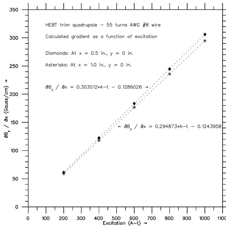
Fig. 6. Calculated gradient as a function of excitation of a HEBT quadrupole with a coil of 55 turns of AWG #8 wire.
