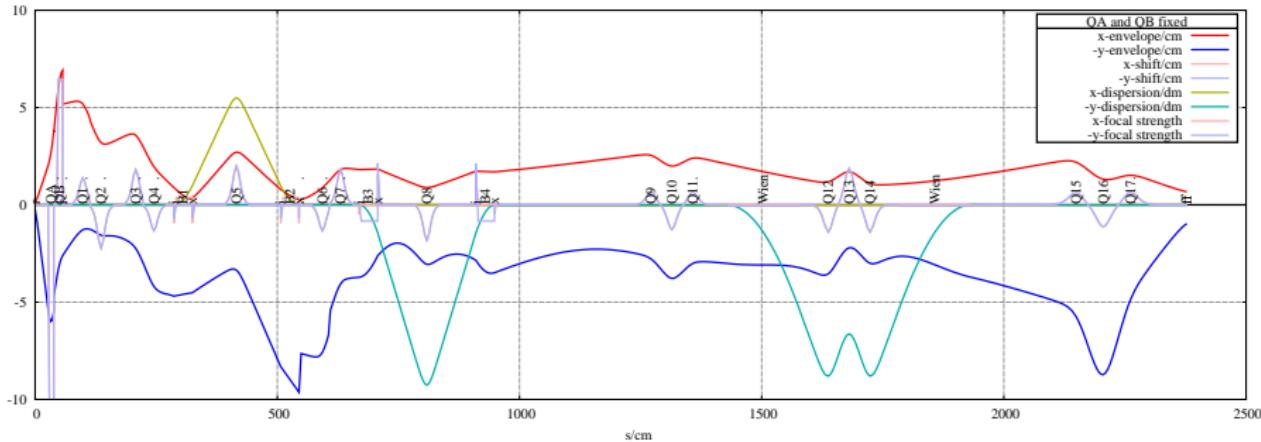
Note that the envelopes are cut by ‘slits’ sized to reflect vacuum chamber:  $x$  is cut at QB, and  $y$  is cut at the dipole B2. This shows that the chosen initial beam just barely fits into the 6-inch beam pipe. Quad strengths are fitted to minimize the cut and meet the fit constraints mentioned above.
