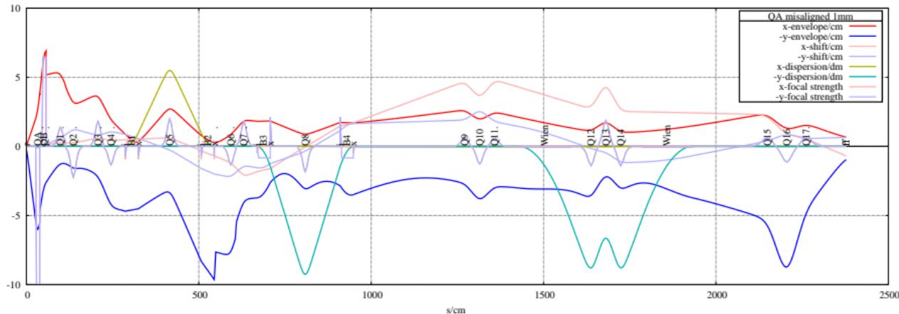
I conclude that there have to be tight tolerances of order 0.1 mm, not only for the placement of the doublet with respect to the beamline centreline and T1, but importantly, the quadrupoles' axes have to be located and fiducialized to the same tolerance. This applies to the quadrupoles individually. The doublet assembly can have an alignment tolerance about 2 to 3 times more relaxed, as long as the tilt angle of the assembly not exceed 0.5 mrad (=0.1 mm/183 mm).
