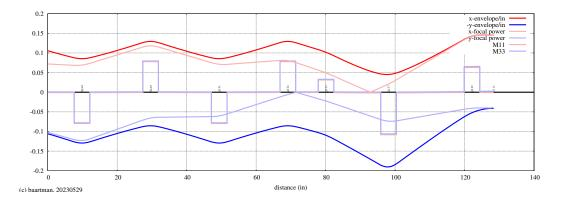
Note that the envelope vertical (y) size is 0.04", or full size of 0.080". This is adequate. The light-coloured traces are the absolute values of matrix elements  $M_{11}$  and  $M_{33}$  calculated backward from the slit. This is to give an idea on where best to apply steering correction, namely, at the locations where this matrix element is small or near zero.
