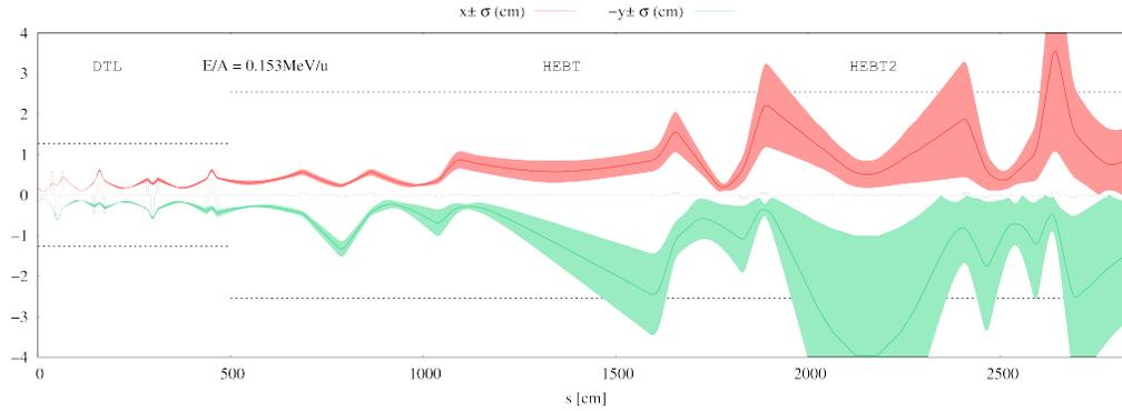
Figure 8: Simulated beam envelopes using TRANSPORT from the DTL to the end of HEBT2. The dotted lines indicate the approximate apertures for each section. A  $\pm 2$  mT deviation is applied to the quadrupoles producing the uncertainty.  $\Delta p/p$  estimated to be between 0.1% to 1%.
