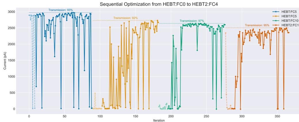
Figure 6: Sequential optimization from HEBT:FC0 to HEBT2:FC4. This covers sequences 2-5, best transmission is shown for each sequence.
