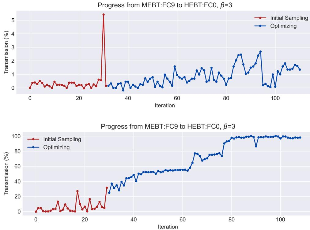
Figure 2: **Top:** Optimization with unbounded quadrupole values. **Bottom:** Bounding quadrupoles to  $\pm 10\%$  of the MCAT value.
