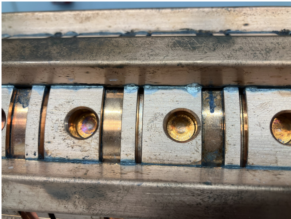
Figure 15: Accelerating cells with hole to manually adjust the field within by force (hammer).
