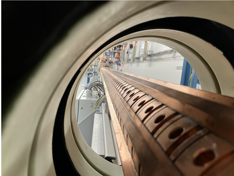
Figure 14: Solenoid around ACC1.
