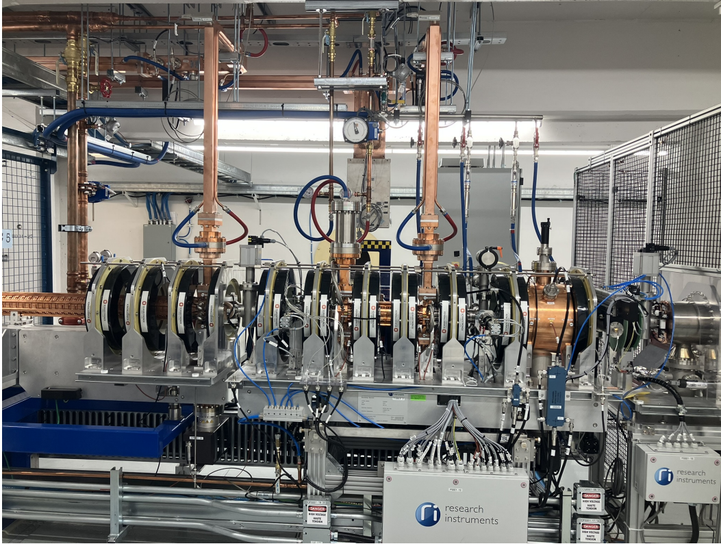
Figure 6: First 3 m from gun (right), with stand alone solenoid (within green plates), pre-buncher (SPB), and the solenoids wrapped around other RF structures (PBU, FBU, ACC1).
