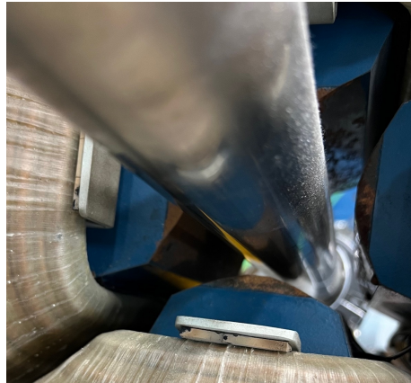
Figure 7: A DanFysik L5 (7.2 mm aperture) at SEBT3B:Q1, with the standard ISAC high energy beam pipe size, showing a noticeable gap between the pole tip and beam pipe.
