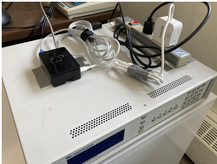
Figure 2: The Raspberry Pi and power bar duct-taped to the top of the Gausmeter.
