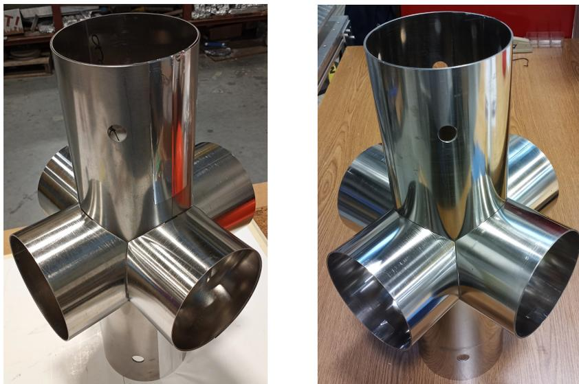
Figure 31: Two mock-ups with identical geometry but different material grade: standard  $\mu$ -metal<sup>®</sup> (left) and Co-NETIC<sup>®</sup>B (right).
